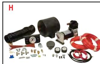
Provides front-to-rear or side-to-side leveling through the use of a dual gauge, heavy duty compressor and 1/2 gallon air tank. This unit inflates each air spring independently (two air springs).
