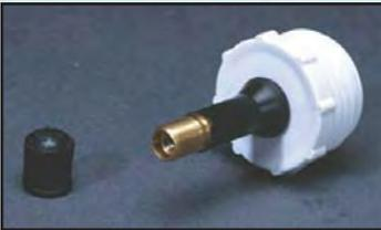
The blow-out plug (27898) has no valve, and is to be used for draining water lines. The blow-out valve (21363) does have a valve, and can be used for draining water lines, as well as for leak tests.
