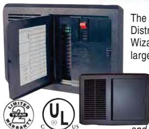
The PD4000 Series "Mighty Mini", is a compact All-In-One AC/DC Distribution Panel and Intel-Power Converter with built-in Charge Wizard®. Compact & lightweight, the PD4000, has front access to a large wiring compartment. The Snap Lock cover stays shut while traveling yet opens with a touch. The AC Distribution Panel is rated for 120 VAC at 30 AMPS. The DC section has up to 12 branch fuse holders. The "Mighty Mini" is available in a 45 AMP model. Dim.: 12.25"W x 8.875"H x 5.625"D.
