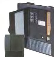
The PD4300 Series AC/DC Distribution Panel has front access to a large wiring compartment and a snap lock cover that stays shut while traveling yet opens with a touch. The PD4300 is rated for 120 VAC at 30 AMPS, is available with either a 45 or 60 AMP Intel-Power converter and features a status indicator and mode control button for the built-in Charge Wizard®. The DC panel accommodates up to 12 branch fuse holders with maximum rating of 20 AMPS each. Dim.: 11.85"W x 14.125"H x 8.5"D.
