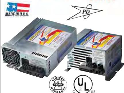
Intel-Power 9200™ Series Converters with BUILT-IN Charge Wizard® will recharge your RV's battery to 90% in 2-3 hours. Many converters only have one charging mode, 13.6 VOLTS, which can result in battery boil-off. The 9200 Series converters have FOUR charging modes: BOOST (14.4 VOLTS), NORMAL (13.6 VOLTS), STORAGE (13.2 Volts) and DESULFATION (13.2 VOLTS with a 15 minute 14.4-VOLT burst every 21 hours).
